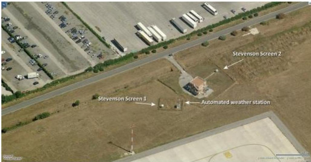
Figure A2: [Ciampino Airport](#) in Rome, Italy. The three thermometers shown get affected by planes, the tarmac, and the truck parking lot.
