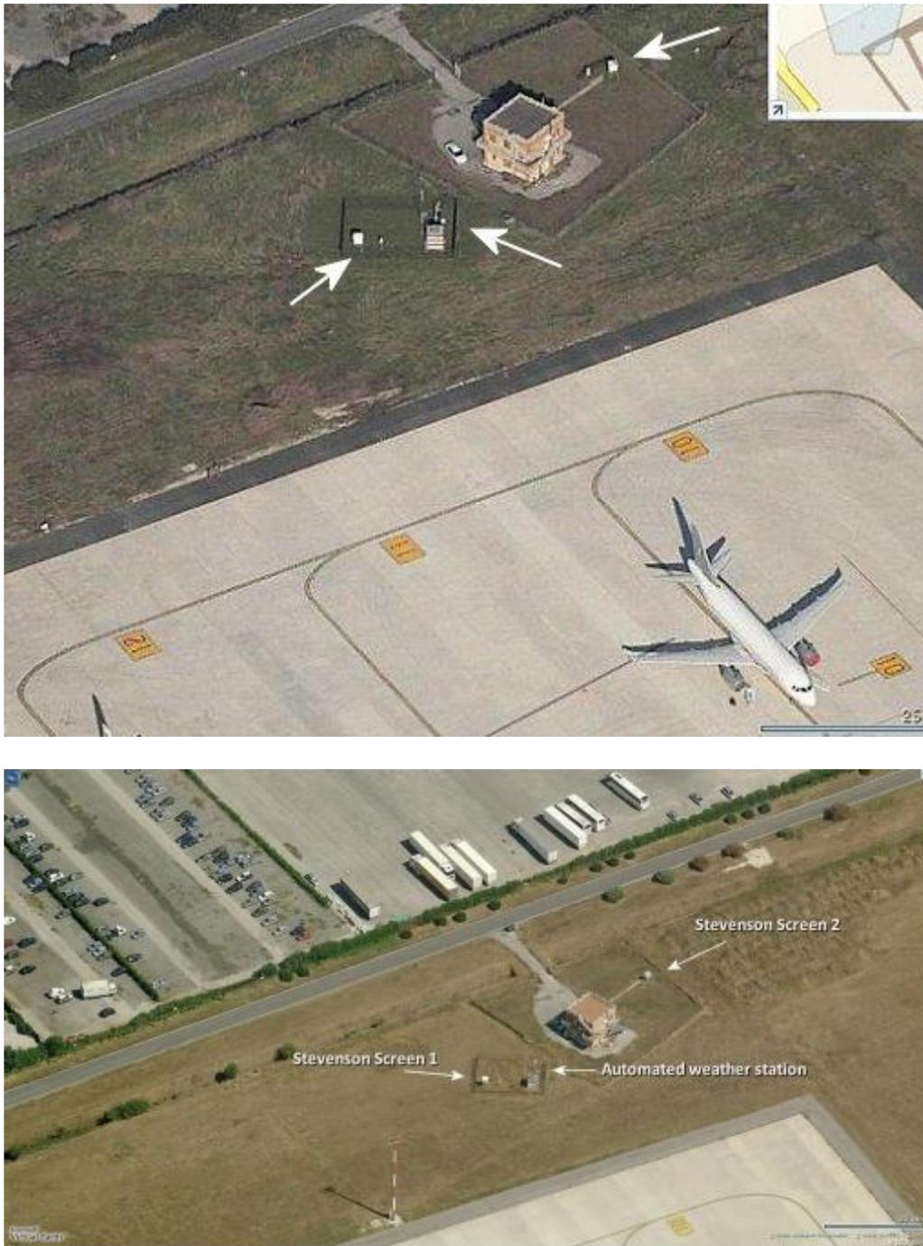
Figure A2: [Ciampino Airport](#) in Rome, Italy. The three thermometers shown get affected by planes, the tarmac, and the truck parking lot.
