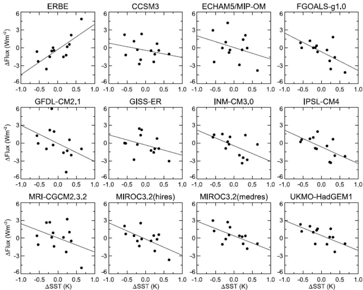
Outgoing radiation from earth (vertical) against sea surface temperature (horizontal), as measured by the ERBE satellite (upper left) and as “predicted” by 11 climate models (the other graphs).
